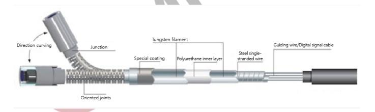
Based on the CMOS image sensor principle, MITECH MVS industrial endoscope can collect picture information in narrow spaces. The digital signal can be transferred to the host through video signal cable plugged in pipe, thus to achieve picture display and storage. The oriented joints connect the probe with insert tube and the guide wire inside the joints can turn 4 directions freely controlled by mechanical device. As a result, the CMOS sensor can shoot excellent photos as required in time.
